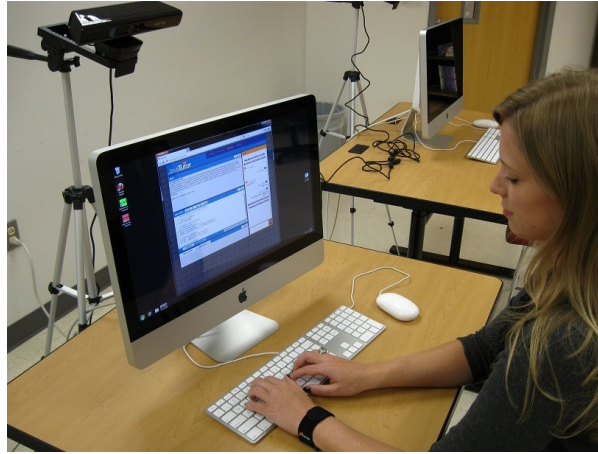
Fig. 2: Multimodal instrumented tutoring session, including a Kinect depth camera to detect posture and gesture, a webcam to detect facial expression changes, and a skin conductance bracelet to detect electrodermal activity.
