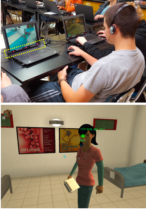
Figure 3: (Top) Students’ gameplay. The yellow dashed box is the Tobii EyeX eye tracker used to capture player gaze traces. (Bottom) Gaze label indicated with green eye icon. The game logs the gaze target’s name in the game trace data. This screenshot was captured for demonstration purposes. Gaze labels are not displayed during gameplay.
