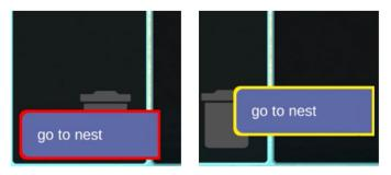
Fig. 7. Observed usability issue when deleting blocks. A block cannot be deleted when it is highlighted in red (Left), and it can only be deleted when highlighted in yellow (Right).
