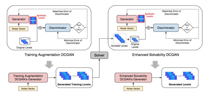
Fig. 4. Overview of the proposed Multistep DCGAN Framework
